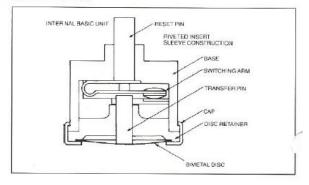
Manual reset snap disk thermostats operate the same way as automatic reset thermostats with one exception. When the snap disk actuates the contact switch, the switch disengages from the disk and does not reset when the snap disk changes back to its original position. The thermostat has a button that is mechanically coupled with the contact switch. Pressing the button physically pushes the switch back to its original position and resets the thermostat.
