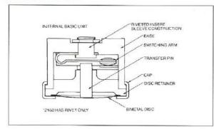
These thermostats are constructed with a temperature sensitive, bi-metal disk which is electrically and thermally isolated from a single pole, single throw switch. This bi-metal disk is slightly convex, but when the temperature reaches its set point, it snaps into a concave shape. Bi-metal snap disks are calibrated to change state and reset at standard temperatures but can be customized to fit specific application temperature requirements.
